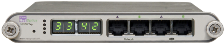
Figure 1 : 33% Utilization of One Side of the Link and 42% Utilization of the Other Side
