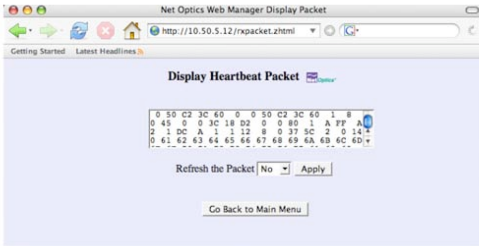
Figure 8: Web Manager displays the current Heartbeat packet values
